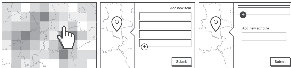
Fig. 2: Simplified process of annotation and creation: 2.1: Identify missing data by e.g. interlacing expert knowledge with the visual blank spots; 2.2 By selecting a region, an interface for annotation or creation appears; 2.3 It is possible to extend existing structures by adding custom attributes
